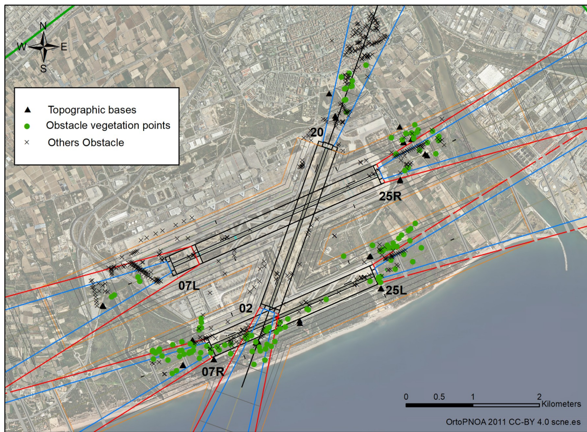
Fig 3. Topographic bases and vegetation obstacles and elements for monitoring. CC-BY 4.0 scne.es 2011.
